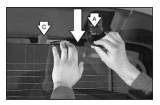
Squeeze and pull down the latch levers (A), located near the upper corners of the rear glass, to unlatch. Once unlatched, the glass-catch release button (C) will catch the rear glass and prevent it from falling forward.
